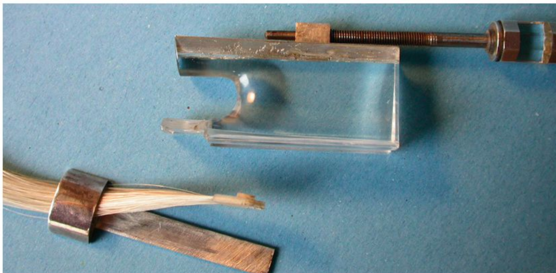
Figure 13. The synthetic barrette in the frog by Gilles Duhaut.
