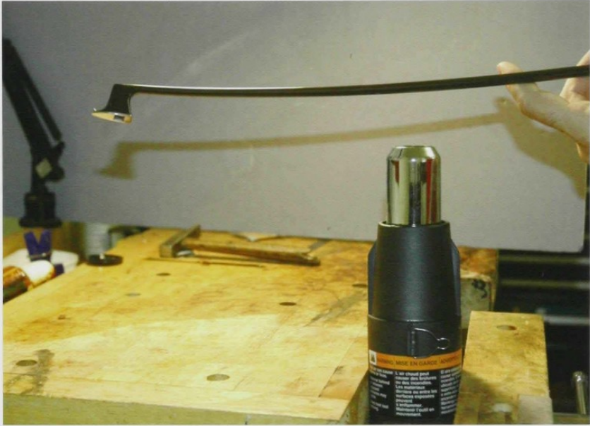
Figure 9. Heating a synthetic stick.
