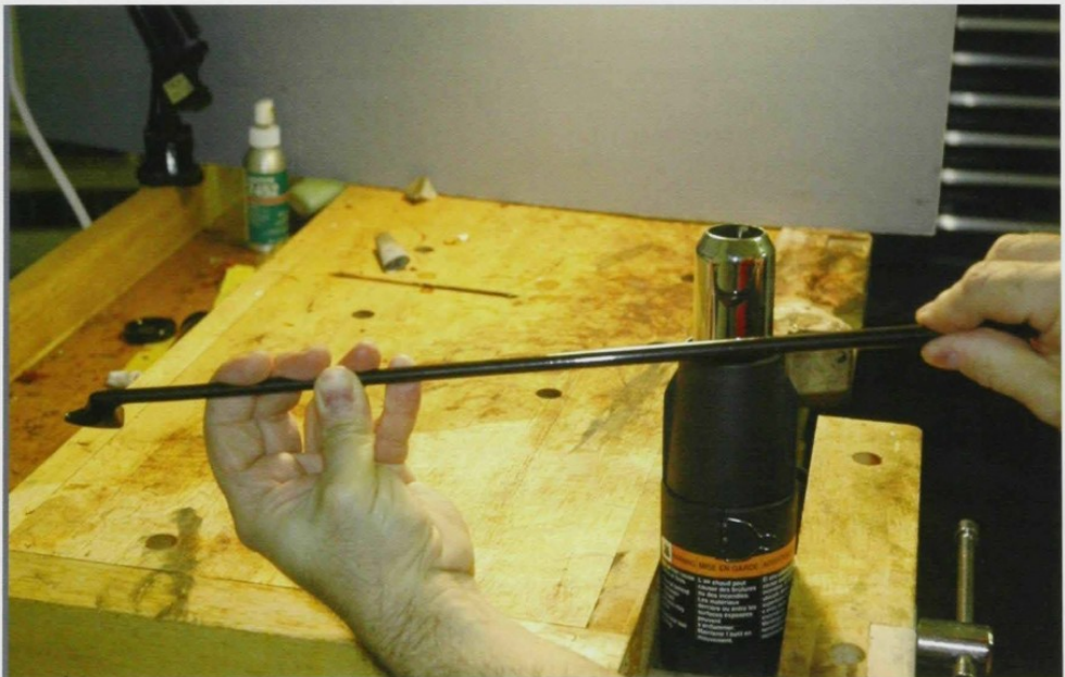
Figure 10. Straightening a synthetic stick.
